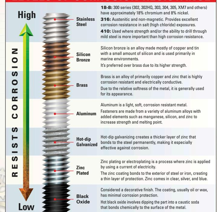
Cold black oxide is a copper selenium compound that is applied at room temperature and tends to rub off easily.
