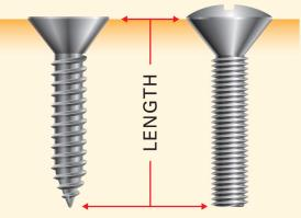
For fasteners that countersink, measure from the point where the head meets the surface material to the end of the fastener.
