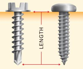
For screws that sit above the surface material, measure directly under the head to the end of the fastener.
