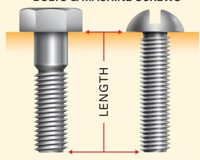
Cap bolts and machine screws that sit above the surface material, measure directly under the head to the end of the fastener.
